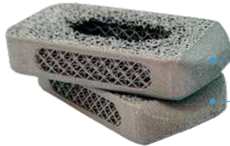
Smooth surface with a downfacing roughness down to 6 \mu\text{m} R_a , after sand blasting
