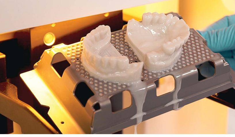
The NextDent 5100 can print a full arch in 30 minutes according to Matt Mills, owner of Hybrid Technologies.
